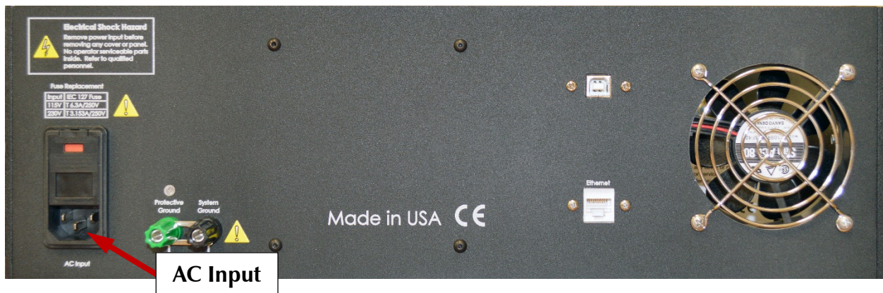
Figure 4-2 Rear Panel of the EIS Box 5000
