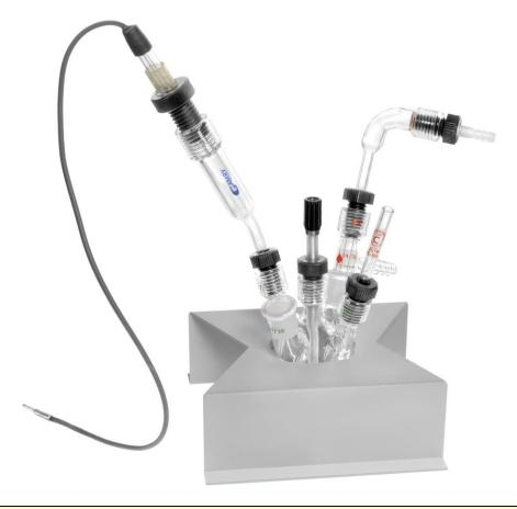
Pay careful attention to cell cleanliness. In most electrochemical testing situations, contaminants in the cell and test solution can lead to poorly reproducible results. If you touch the cell components with your fingers, you can inadvertently add salts and organic compounds to your cell solution. We recommend that you carefully clean the cell components using good laboratory practice. After the components are clean, avoid touching their wetted surfaces.
