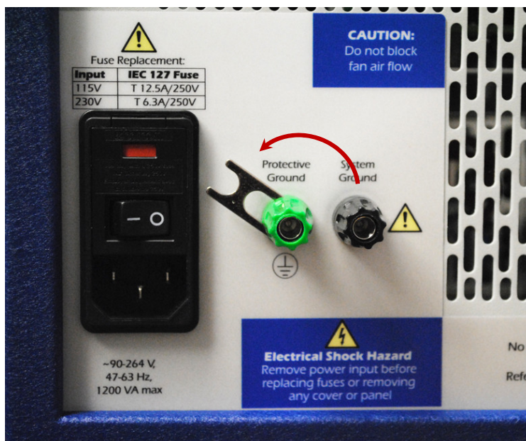
Figure B-4 Storing Ground Jumper When Disconnected
