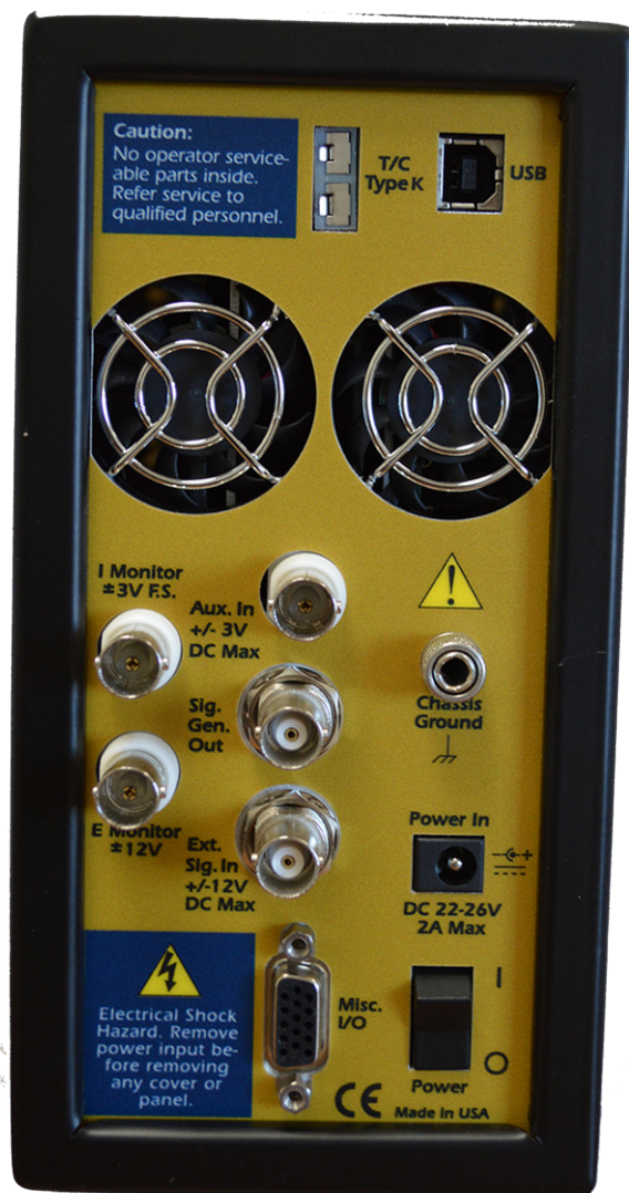
Figure 4-2 Rear Panel of the Reference 620
