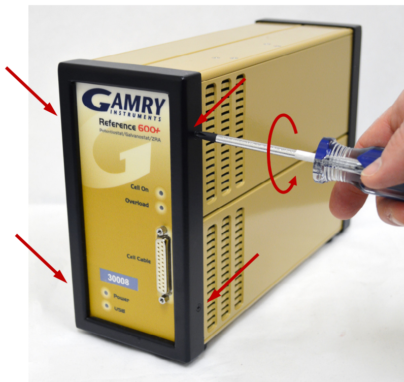
Figure 4-5 Removing the Front Bezel
