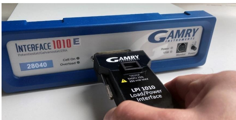
Figure 4-2 Installation of the LPI1010 D-sub Module at the front of an Interface 1010 potentiostat
