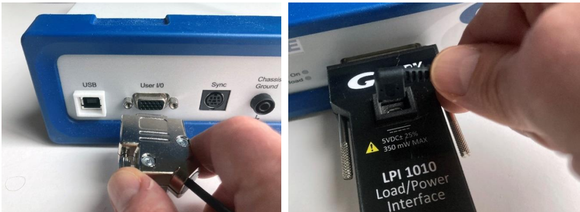
Figure 4-4 Installation of the LPI Power Cable at the rear of an Interface 1010 potentiostat (left) and USB-C connector of the LPI1010 D-sub Module (right)
