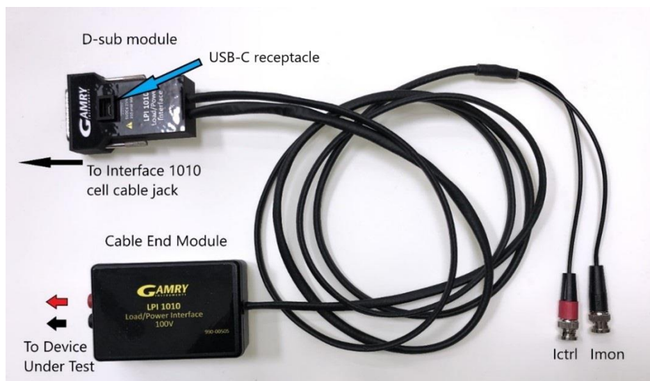
Figure 3-1 Overview of the LPI1010 Top-Level Assembly
