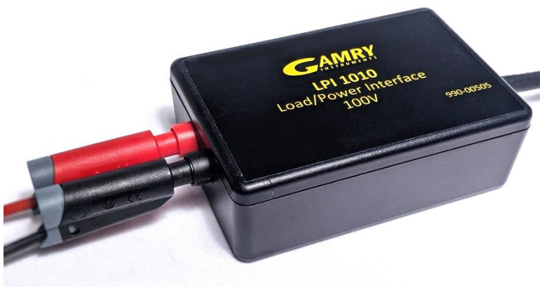
Figure 4-7 LPI Voltage Sense Cables connected to the LPI Cable End Module
