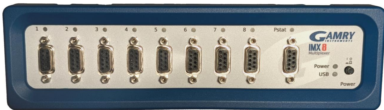
Figure 3-1 Front View of an IMX8 Multiplexer
