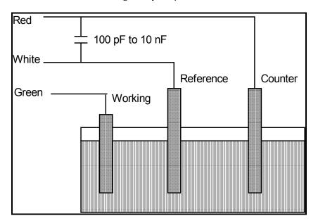
• Add resistance to the counter electrode lead. See Figure 4-3. This change lowers the effective gain bandwidth product of the control amplifier. As a rule of thumb, the resistor should be selected to give one volt of drop at the highest current expected in the test being run. For example, if you expect your highest current to be around 1 mA, you can add a 1  $k\Omega$  resistor.
