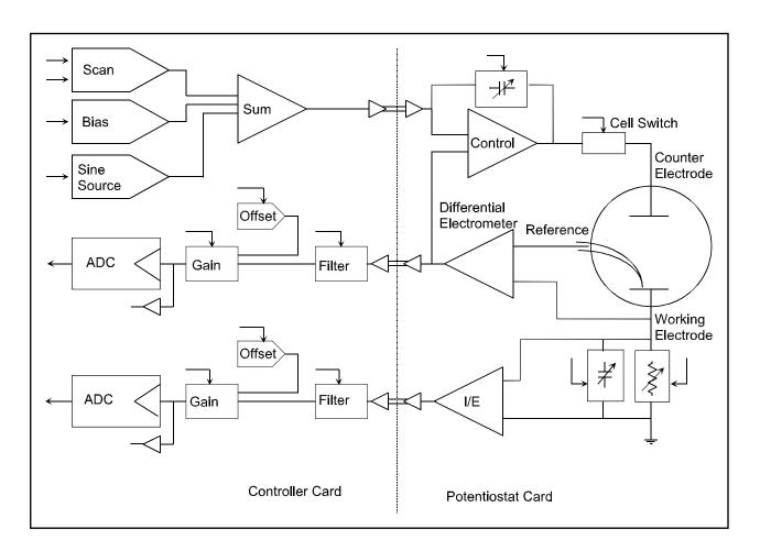
Figure 1-1 PC4 Analog Circuits in Potentiostat Mode
