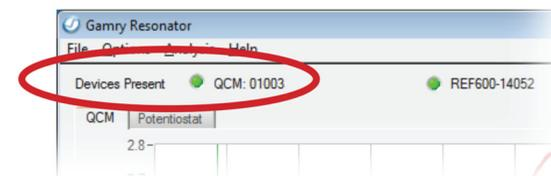
The green indicator indicates successful connection, your device is ready to use. Please refer to the eQCM 15M Operator's Manual for detailed information on the various indicator states.
