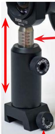
Equalize heights of LED and photodiode using scales on optical posts. Align LED and photodiode to center of cage posts.
