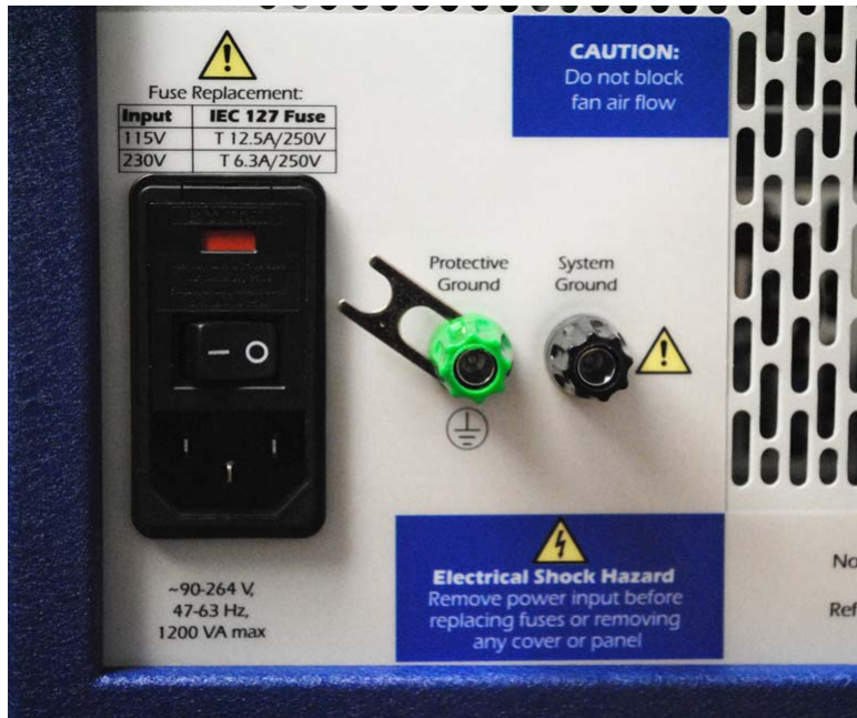
Figure B-2 Storing Ground Jumper When Disconnected
