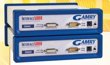
The Interface 5000 is designed for testing of batteries, supercapacitors, and fuel cells. There are two versions available, the 5000P which provides capabilities for typical testing of single cells using techniques such as charge, discharge, cyclic charge/discharge, potentiostatic, galvanostatic, and galvanostatic EIS to 20 kHz. The 5000E includes Gamry's full suite of electrochemical techniques and extends the impedance frequency range to 1 MHz.
