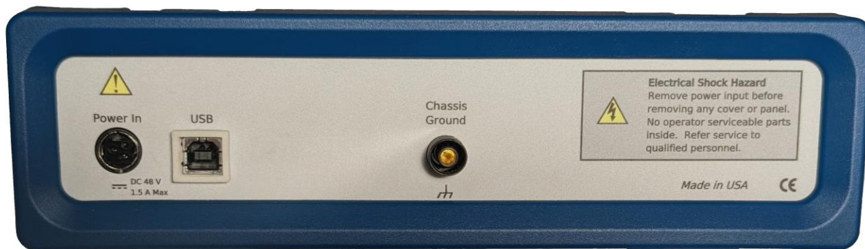
Figure 3-2 Rear Panel of the IMX8 Multiplexer
