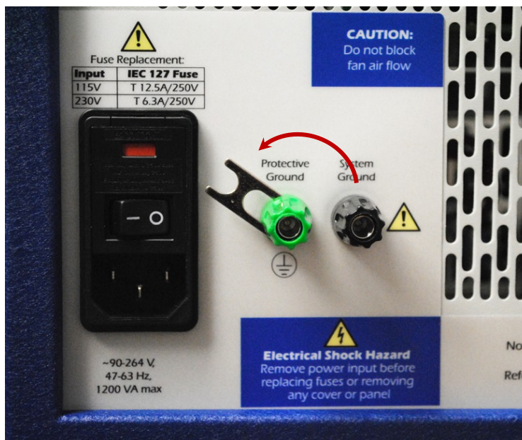
Figure B-4 Storing Ground Jumper When Disconnected
