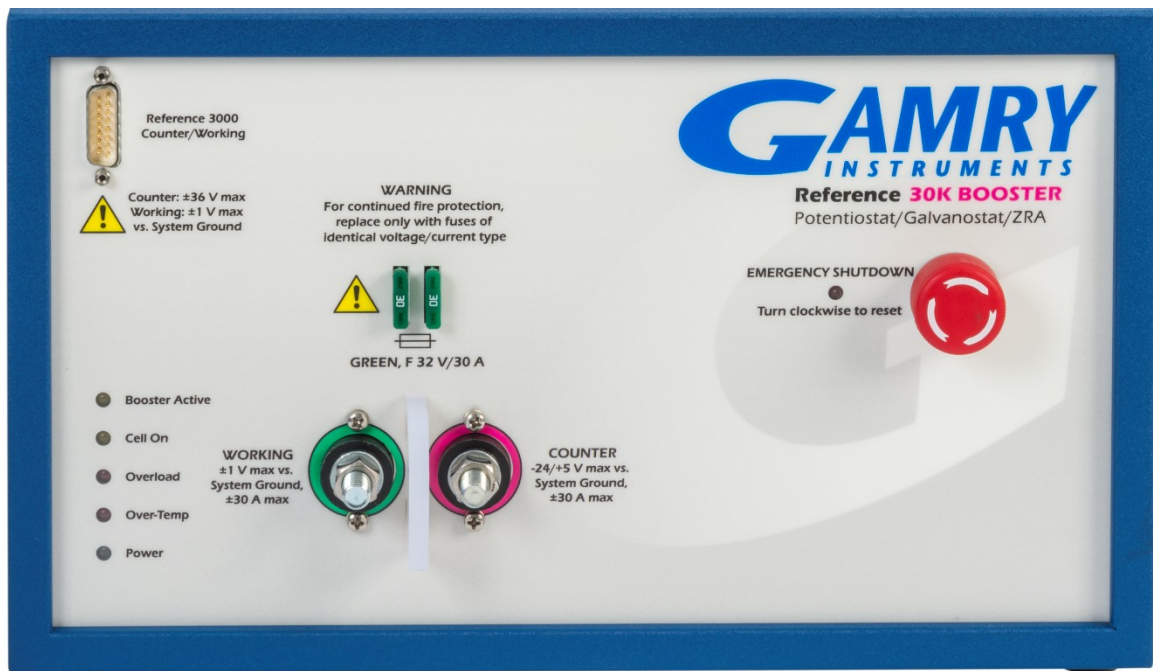
Figure 4-1 Front Panel of the Reference 30k Booster
