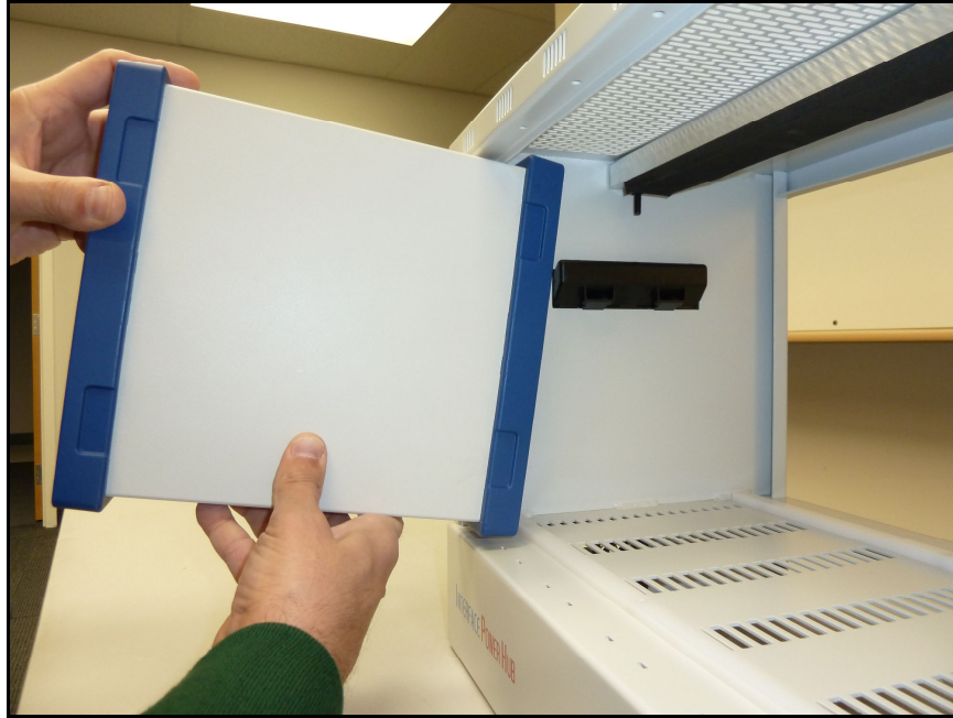
Figure 3 - 6 Tilting the Instrument to Place it in IPH Chassis
