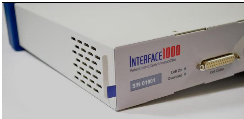
Figure 3-10 Instrument with Bezel Removed - Label Tab Seen
