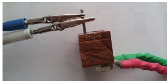
Figure 1 – Shorted lead test fixture. Sense leads are connected at top, current leads at bottom.
