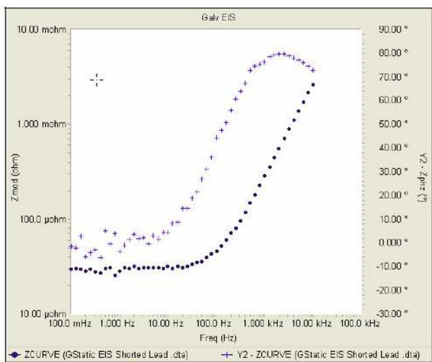
This spectrum fits well to a series RL model with a resistance of 30 μΩ and inductance of 42 nH. The resistance value is interesting. The copper braid used to make the shorted connection has a measured resistance of 8.4 μΩ per mm. 30 μΩ corresponds to a path of 3.6 mm through the braid.
