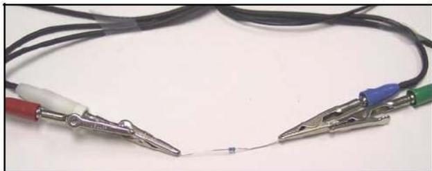
Record the potentiostatic EIS spectrum of this resistor with zero DC and 20 mV<sub>rms</sub> AC voltage. The frequency range should extend from 0.2 Hz to the system's maximum specified frequency.
