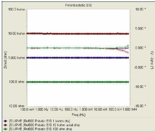
The magnitude of an ideal resistor's impedance is independent of frequency and the phase is zero.
