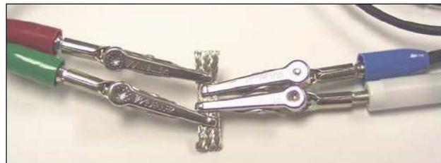
The Working Sense and Reference leads are the inside pair of connections. Don't allow the clip leads to touch except at the braid connections.
