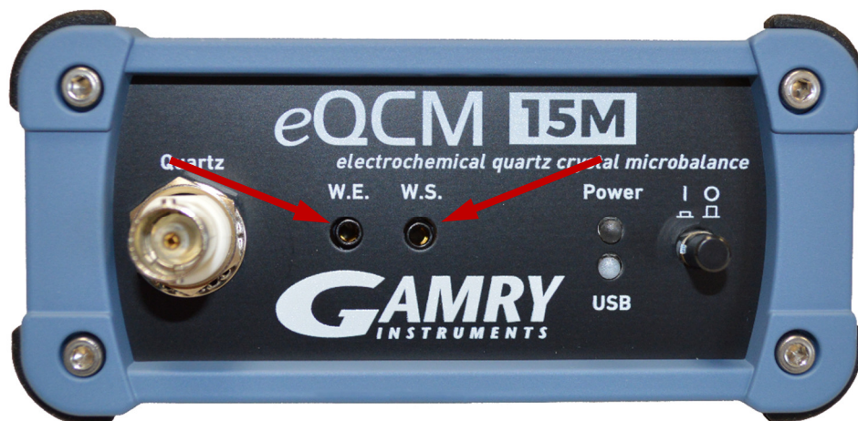
Figure 5-2 Connection of Working (Green) and Working Sense (Blue) Leads to eQCM 15M
